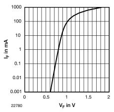
Fig. 4 - Typical Forward Current I<sub>F</sub> vs. Forward Voltage V<sub>F</sub>
