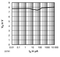
Fig. 5 - Typical Reverse Voltage  $V_{\rm R}$  vs. Reverse Current  $I_{\rm R}$
