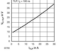
Fig. 7 - Typical Clamping Performance at 100 ns Transmission Line Pulse (TLP)
