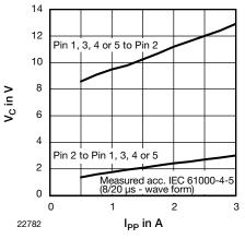
Fig. 6 - Typical Peak Clamping Voltage  $V_C$  vs. Peak Pulse Current I<sub>PP</sub>
