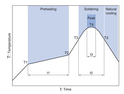
Preheating Soldering Peak Temp. Time Temp. Time Temp. Time T1 T2 T4 Т3 t3 150°C 180°C 90 to 120s 230°C 255°C 10s max. 40s
