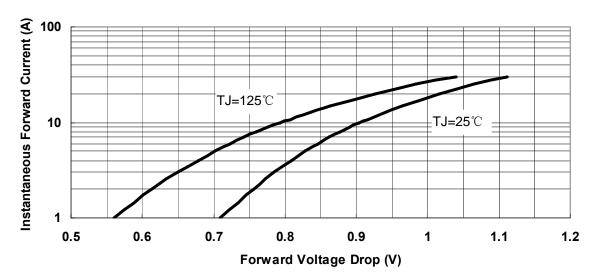
Fig.3-Typical Instantaneous Forward Voltage Characteristics
