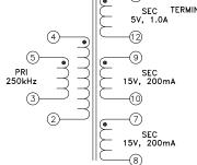
Application of the transformer requires terminals 4&5 and 3&2 be internally connected on the PCB.
