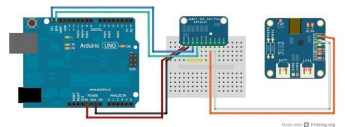
All input signals to these devices must be between ground potential and VCC. If your
